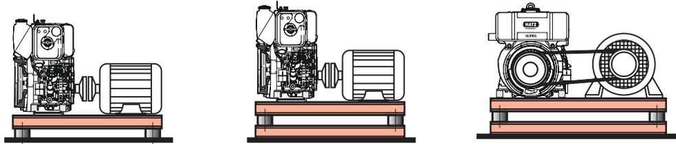
When systems are mounted on a single-axle trailer with rubber tires, the engine must be mounted over the axle.
