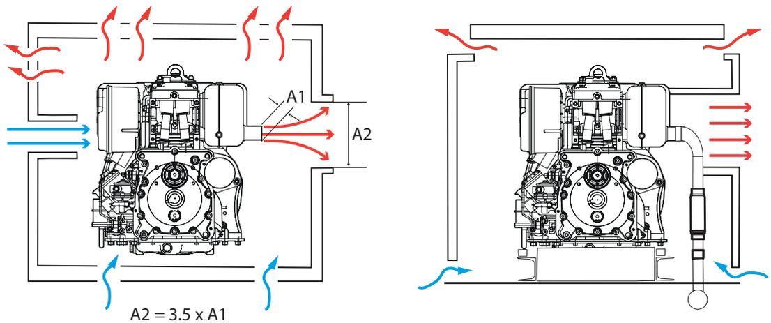
The openings for the radiation heat must be arranged in such a way that a chimney draft occurs that carries away the heat energy. Exhaust silencers must be installed outside of the cover and the exhaust pipe must be routed along the shortest possible path out of the cover. The radiation heat of the driven machinery, such as hydraulic pumps, must be able to escape as well.
