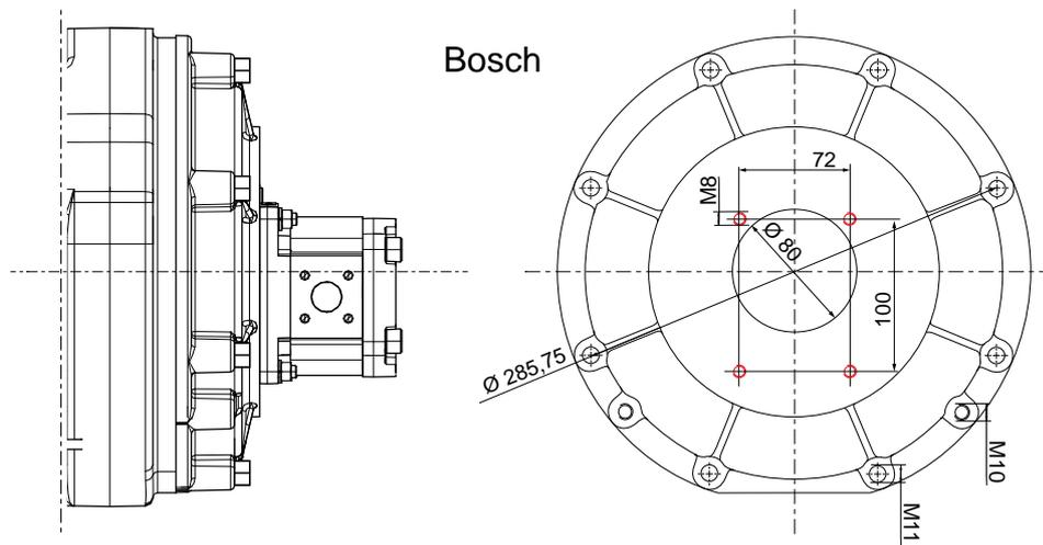
Installation option on the flywheel side on the connection housing for engine types 1D50, 1D81, 1D90, 1D90E
