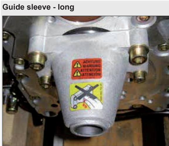
If a warning label on the engine is concealed (e.g. by a cover, encapsulation, etc.), the machine must be checked to determine whether the danger still prevails. If the danger has been eliminated, the additional warning label can be omitted. If the danger persists, a new warning label must be applied by the machine manufacturer. Thus, the machine manufacturer is responsible for the correct application of the warning labels on the engine and on the machine.
