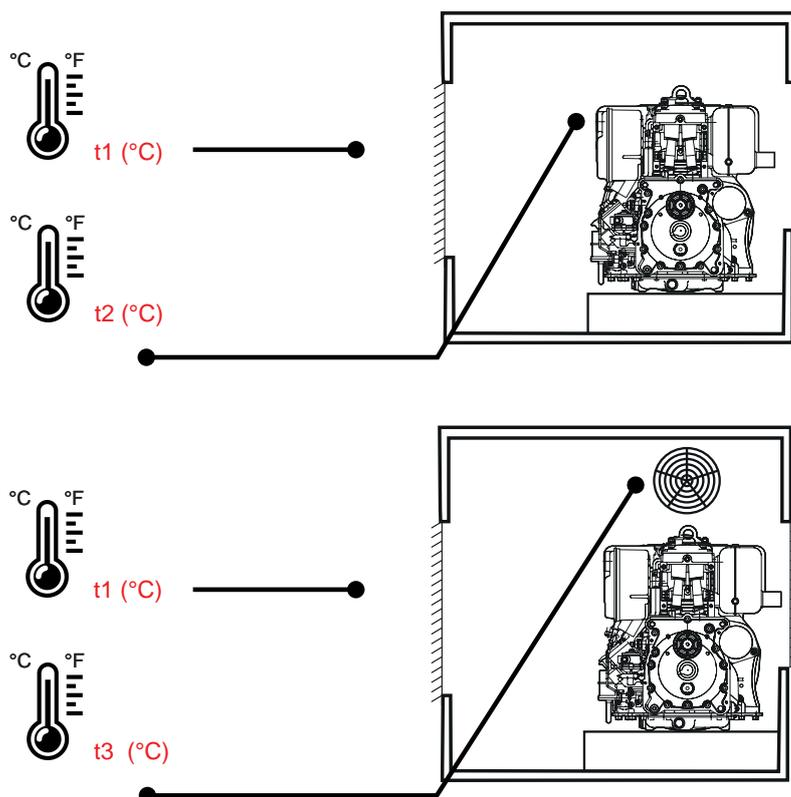
A temperature increase, of course, overrides the normally applicable temperature limits. This means that at a temperature increase between the outside air and the intake air of 8 to 10 °C, the engine can no longer be operated up to the ambient temperature of +45 °C but now only up to approx. 35 – 40 °C.
