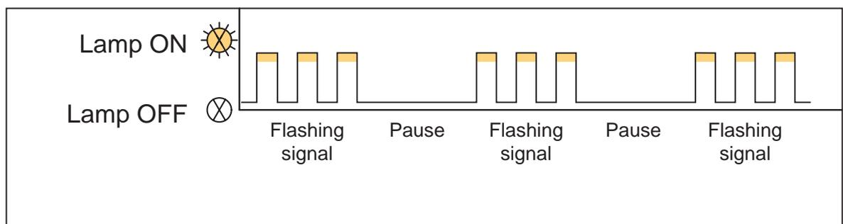
The light flashes three times in a row for each error. If two or more errors are active, these are flashed immediately afterwards. To repeat, turn the starting key to position "0" and then back to position "I". The flash code is deleted automatically if the error does not reoccur within two operating cycles (= start/operation/stop).
