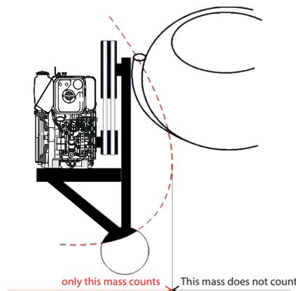
Only sufficiently large masses in the direct vicinity of the engine can prevent strong vibrations and possible material breakage.
