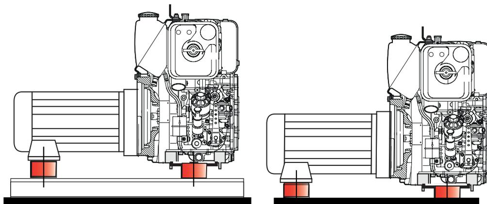
A U 80 profile (vertical) is adequate for the frame parts of a flexibly supported and flange-mounted force sensor, since the flange-mounted power take-off is stiff and cushioned by the rubber buffers. To stabilize the flexibly supported machine during the starting and coasting phases, stable rubber buffers must be used under the machine part with low vibration (e.g. generator).
