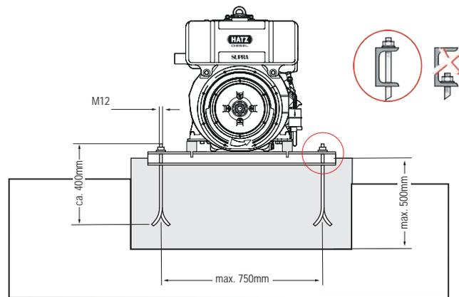
The anchor bolts used for fastening must be approx. 400 mm long. A size M12 cross section is recommended. The anchor bolts must be screwed through the U profile (see figure); this ensures a level washer and nut contact surface and the necessary bolt preload.
