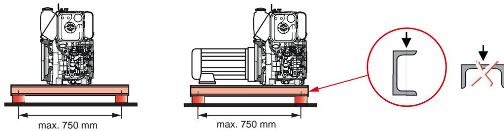
The dimensions recommended above for the rolled U profile only apply for vertically erected U profiles. The necessary stiffness is only achieved in this position.
