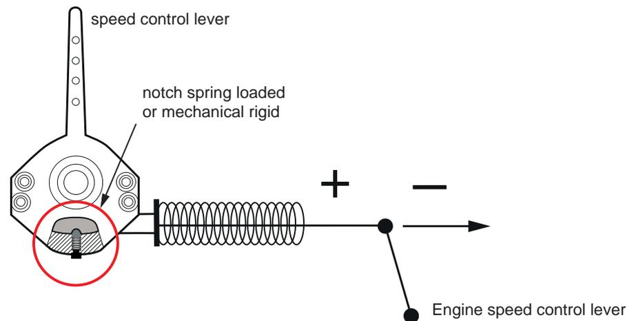
The Bowden cable lever is locked in the position of the operating speed (by a flap, a ball with spring force, etc.).
