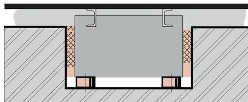
Building of the foundation must be commissioned with a construction company that provides a guarantee that the foundation is properly constructed. The foundation block is seated on ground with a sufficient load-bearing capacity.
