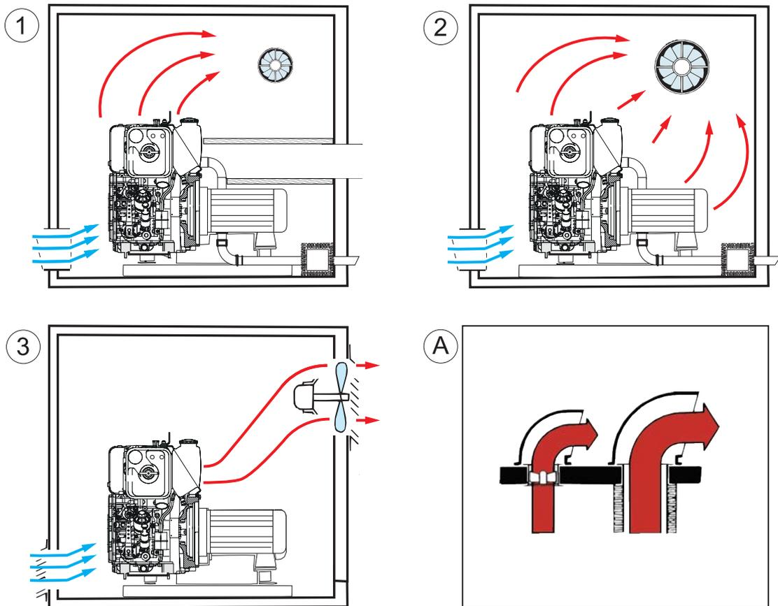
The **outlet openings** of the air outlet ducts and the exhaust air fans must always be installed on the building side facing away from the usual direction of the wind. If wind blows into these openings, the air current will be blocked and the temperature level in the machine room will rise to impermissible levels.
