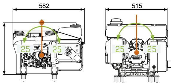
\* Max. tilt position [°], dimensions [mm]
