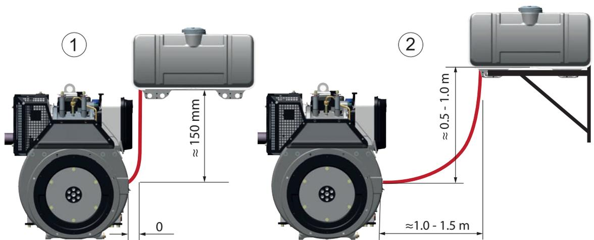
A fuel pump is necessary if the tank is lower (1) than the filter and injection pump. Even at an in-feed line length of approx. 1.5 m and with the tank located higher than the engine (2), a fuel pump (standard for 1D90E) is necessary to overcome the line resistance, or the line cross section can be enlarged.
