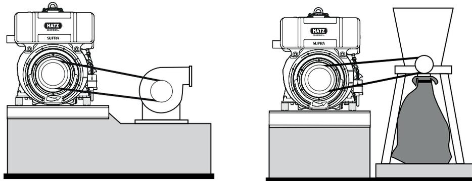
To isolate vibrations and structure borne noise from buildings, concrete foundations should be separated from the buildings by means of springy mats or similar in case of high speeds – i.e. they should be flexible and thus insulated against structure-borne noise.
