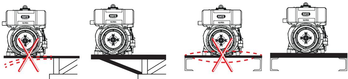
If frame parts are longer than 750 mm for structural reasons (e.g. engines with multistage pumps), these must be bolted down again after a maximum distance of 750 mm.
