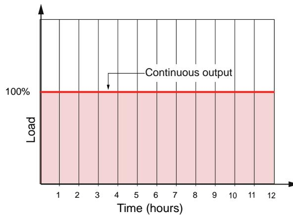
This power setting is used, for example, for irrigation pumps and for machines that can be run on the torque rise curve for hours (e.g. joint cutters at maximum feed).
