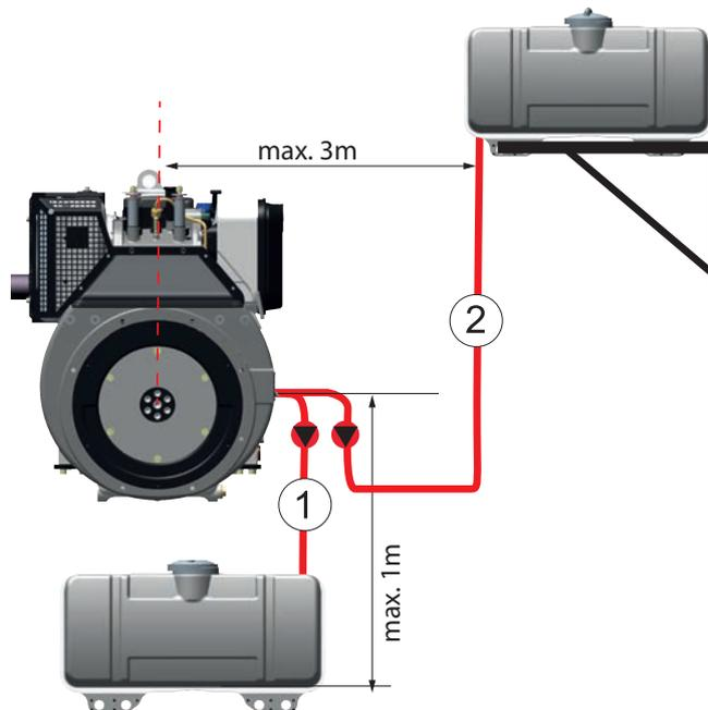
When using a fuel pump with a fuel tank that is not installed at the engine, the fuel filter and the fuel lines must be installed in a way that enables them to be bleedable.
