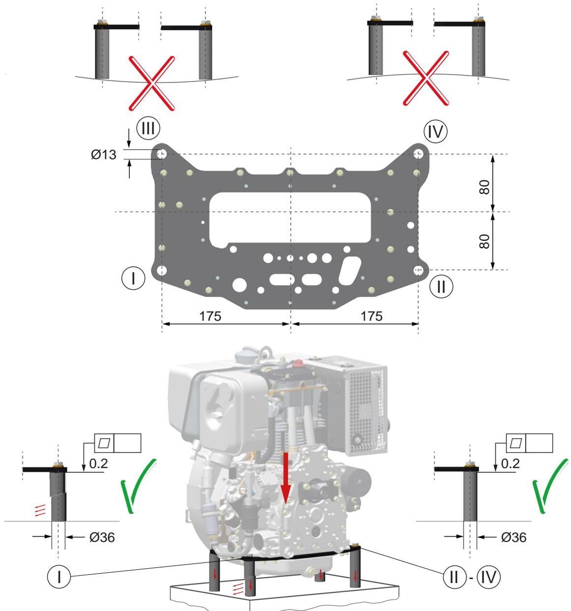
In order for the engine to be installed absolutely free of stress, one of the spacer bushings (I) must be adjusted/aligned to the contact surface.
