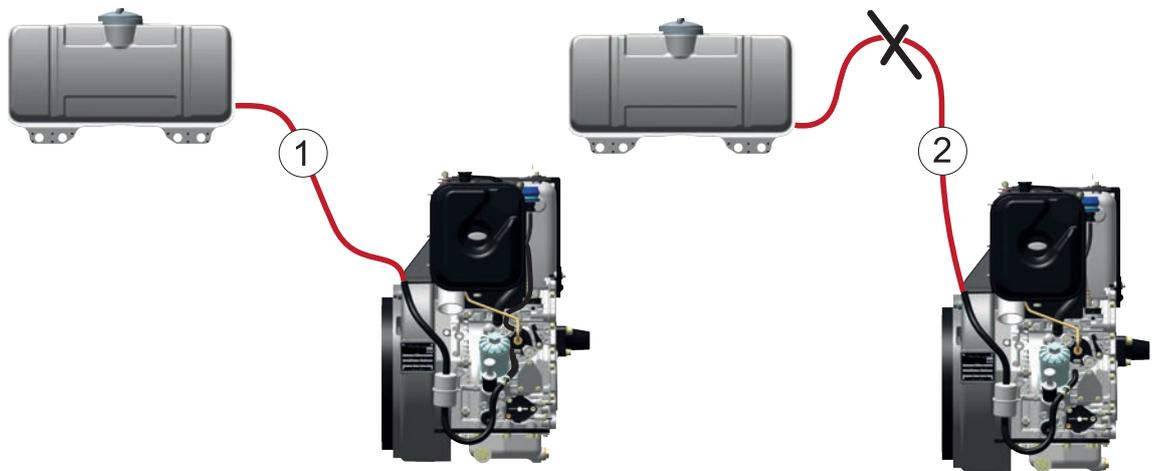
If the fuel tank is installed on the wall and not at the engine, a gradient of 0.5 – 1.0 m must be maintained to overcome the line resistance. If the fuel tank is in the immediate vicinity of the engine, a gradient of approx. 150 mm between the tank outlet and the injection pump is usually sufficient.
