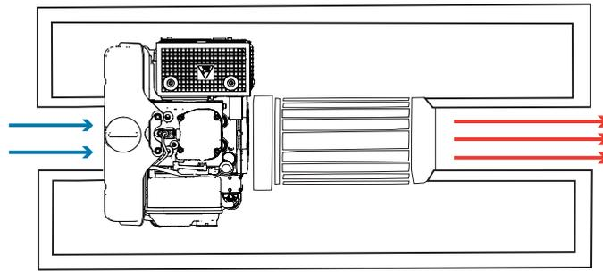
The opening area in the trim panel must be approx. three to five times as large as the discharge area at the cylinders and cylinder heads. The opening in the cover should have guide plates.
