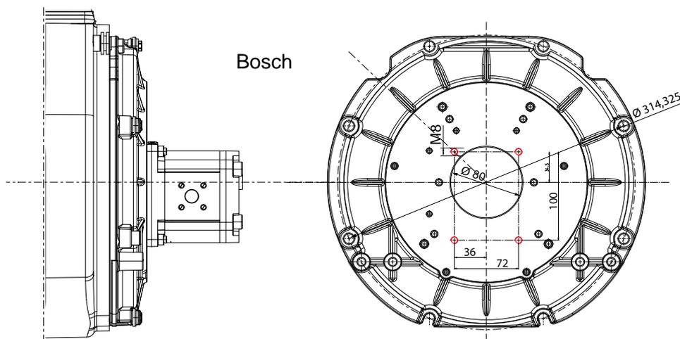
Depending on the model size of the hydraulic pump (HP) and the associated connection shaft, an additional connection ring for the SAE-A, SAE-B or SAE-Bosch connection housing must be used when installing an HP for the engine specifications 1D50 and larger on the SAE 5 engine connection housing ( $\varnothing 314$  mm).
