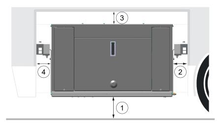
The following minimum distances around the system must be observed when installing it in a vehicle.
