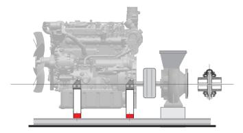
In contrast, variants I and II are not permitted because the engine and machine form separate vibration systems which work against each other and damage the flexible coupling or belt.
