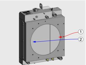
Measuring positions on cooler, engine side, pressure fan
