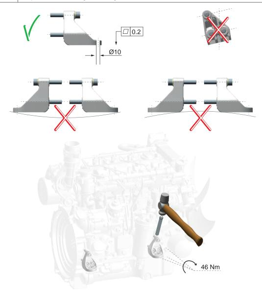
Tightening torque of engine bracket M10 with 46 Nm. In order for the engine to also be installed absolutely free of stress, one of the 4 identical engine brackets must be adjusted/aligned to the contact surface.
