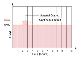
The engine setting takes this overpower capability into account. The magnitude of the overpower is selected depending on the purpose of the engine – normally it is set to an overpower of 10%.
