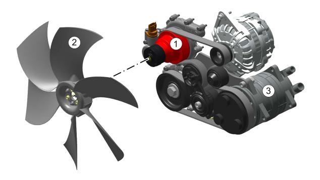
• The **raised (3)**\* fan mounting position is equipped with reinforced bearings like the version with boosted water pump: The mounting weight of max. 5 kg tested and approved by Hatz, with unbalance class G2, also applies here.
