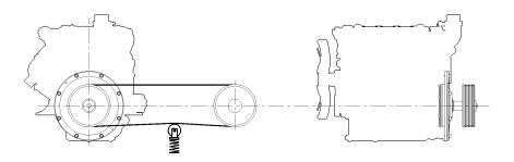
The actual force effect in case of flexible belt tension can be calculated as follows:
