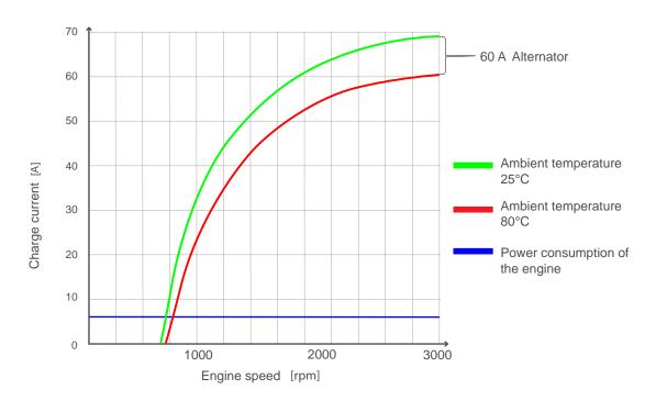
The power consumption of the engine is an approximate value that depends on multiple conditions (such as temperature, voltage, etc.). The starting procedure consumes approx. 1 Ah.
