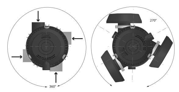
Permissible tilt positions of dust discharge valve
