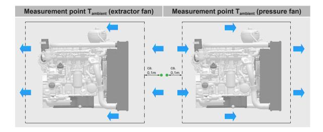
The temperatures are determined with the machine operating at full load, where the coolant liquid thermostat must be bridged (widened thermostat with full opening). With the exhaust fan, the air temperature is determined at the cooling air inlet in the engine compartment.
