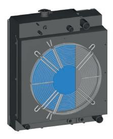
Maximum coolant temperature  $T_{\text{max}}$  is 105 °C. The (standard) engine cooler from HATZ is a heavy-duty version and usually does not require a coarse dirt mesh. This is not to be confused with the contact guard for the fan. The contact guard can be provided by HATZ.
