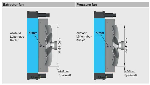
Standard ratio  $\mathbf{n}_{fan} = 1.116 * \mathbf{n}_{engine} [1/min]$
