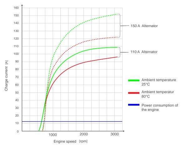
The power consumption of the engine is an approximate value that depends on multiple conditions (such as temperature, voltage, etc.). The starting procedure consumes approx. 2 Ah.
