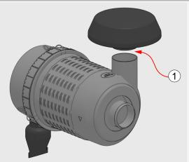
Measuring position (1) at the air filter intake, intake temperature
