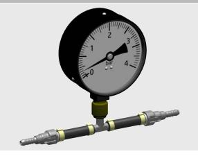
Connect pressure gage between return on engine and return line. See also 8.5.3 fuel circuit diagram, page 90 pos. 9.
