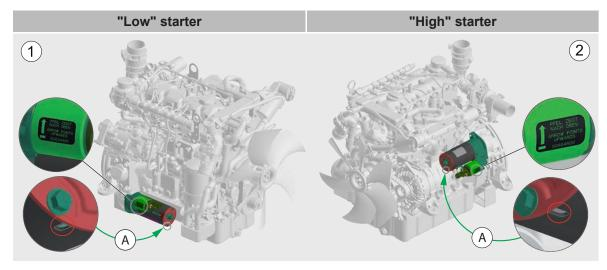
With the ignition switch, the pull-in winding and holding winding of the starter solenoid (terminal 50) (1) are switched on via the starter relay (short-term max. **56 A** in the pull-in winding and **10 A** in the holding winding).
