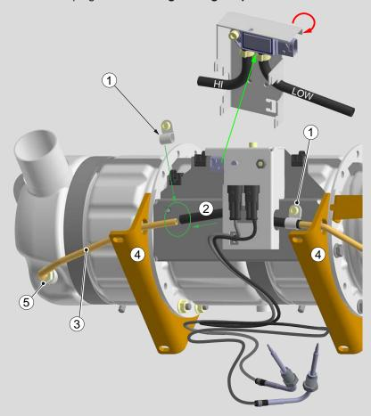
Ensure that the **high pressure (HI)** side is connected to the pressure pipe at the DPF inlet and the **low pressure (LOW)** side is connected to the pressure pipe on the DPF outlet.
