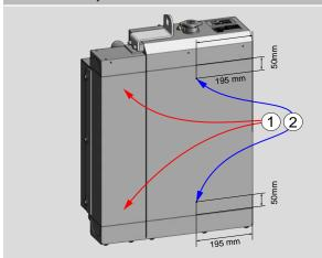
Measuring positions on the cooler on the front of the extractor fan
