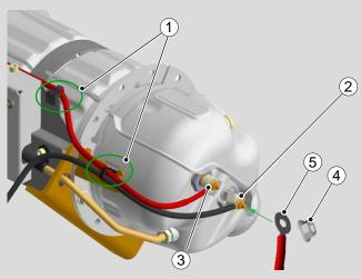
In the 24-V model, the two glow plugs are connected in series.
