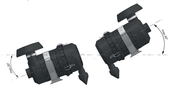
Permissible tilt positions for air intake with and without a rain cap
