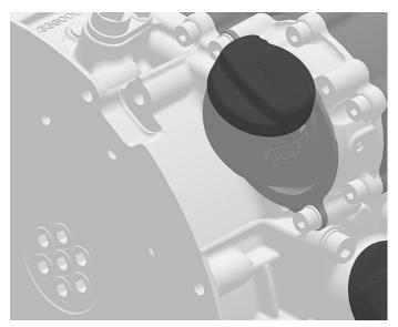
To enable the top PTO to be supplied with pressure oil, the set screw M6x10 must be removed. Failure to do so can lead to **serious engine damage**!
