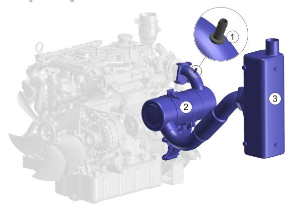
\*Exhaust back pressures apply to the DOC (2) and rear silencer (3) at the measuring point (1).
