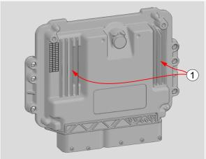
Measuring positions (1) on control unit ED-C17C81
