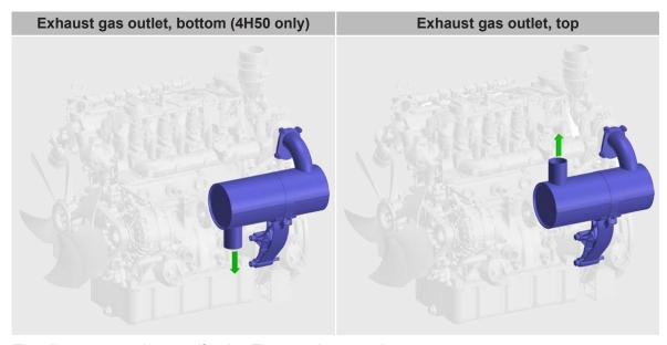
The silencer on engine specification TI cannot be rotated.
