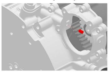
The PTO may only be mounted on CP4 after the pressure oil hole is open.
