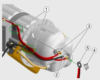
In the 12-V model, two glow plugs are connected in parallel.
